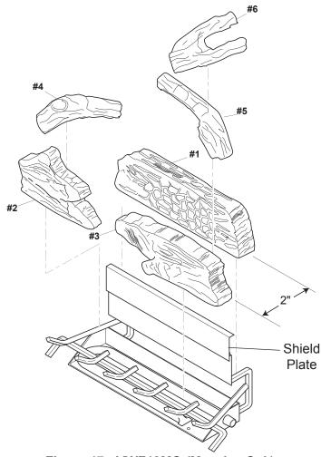
Figure 17 - VWF18MO (Massive Oak) Log Placement
