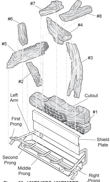
Figure 26 - VWF24SRO, VWF30SRO and Prong VWF36SRO (Split River Oak) Log Placement
