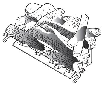
Figure 25 - VWF24B (Birch) Log Placement
