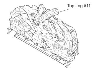
Figure 21 - VWF36MO Log Placement (Massive Oak)
