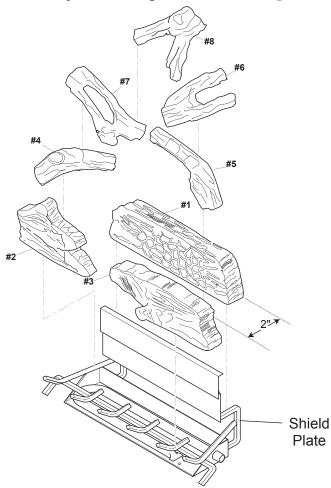
Figure 19 - VWF30MO (Massive Oak) Log Placement
