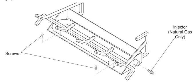
Figure 5 - Securing Grate/Burner Assembly into Firebox
