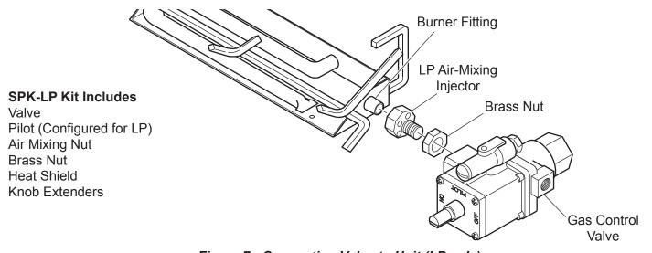
Figure 7 - Connecting Valve to Unit (LP only)
