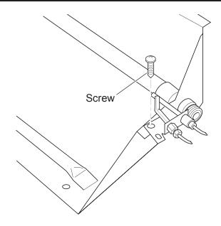
Figure 8 - Installing Pilot
