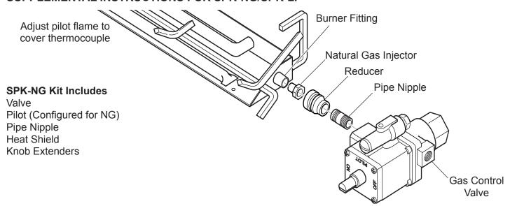
Figure 6 - Connecting Valve to Unit (Natural Gas only)
