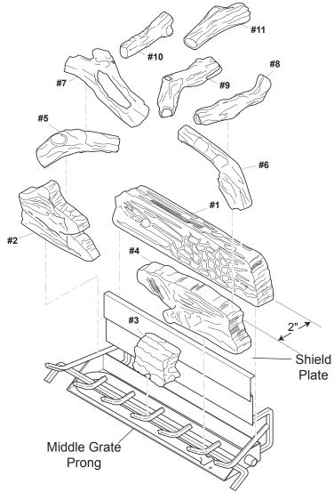
Figure 20 - VWF36MO Log Placement (Massive Oak)
