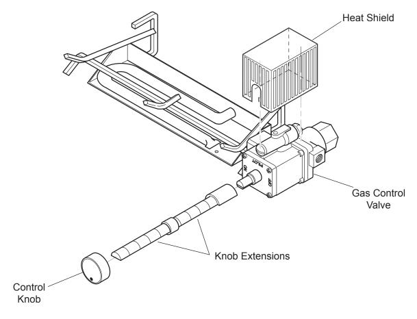
Figure 9 - Installing Heat Shield
