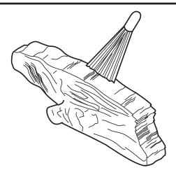
Figure 38 - Removing Soot with a Soft Bristle Brush
