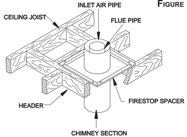
INSTALLATION OF FIRESTOP-SPACER AT FLOOR LEVELS
