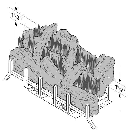
Figure 23 - Correct Appearance of Rear Flames
