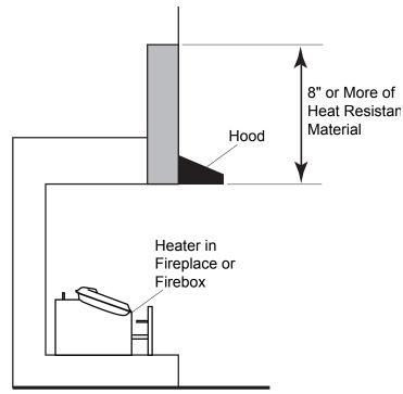
Figure 6 - Measuring Heat Resistant Material for Mantel
