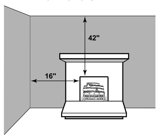
Figure 4 - Sidewall and Ceiling Clearances
