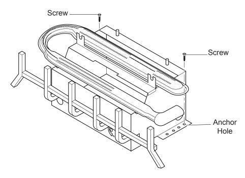
Figure 12 - Securing Heater to Floor of Fireplace/Firebox
