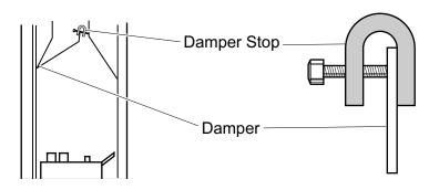
Figure 11 - Damper Stop Installation. (See WARNING at top of next page.)
