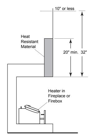
Figure 8 - Minimum Mantel Clearance with No Hood
