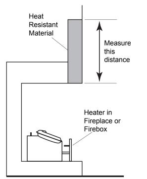
Figure 5 - Measuring Heat Resistant Material
