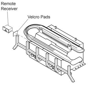
Figure 17 - Installing Remote Receiver
