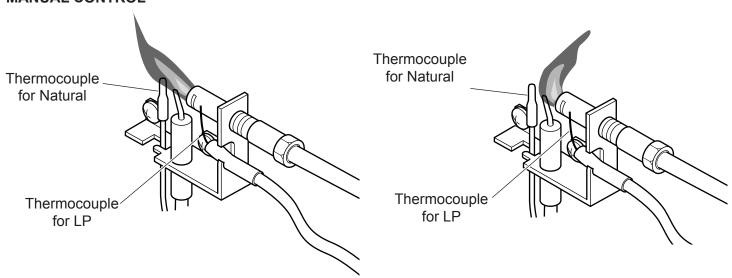
Figure 21 - Correct Appearance of Pilot Flame
