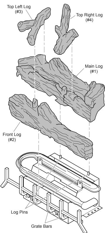
Figure 18 - Installing Logs to Grate
