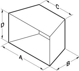
Figure 2 - Hearth Minimum Dimension for Solid Fuel Burning
