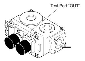
Figure 15 - Pressure Test Point Location Millivolt Control
