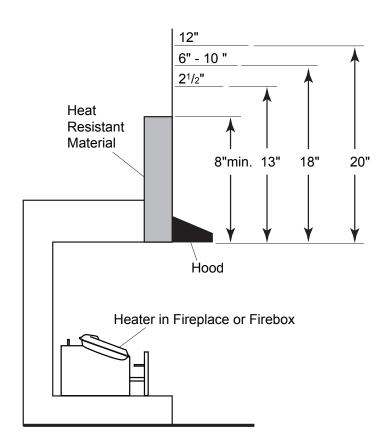
Figure 7 - Minimum Mantel Clearance with Hood
